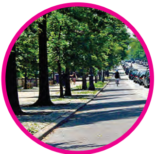
SIDEWALK BUFFERED FROM CYCLE TRACK
