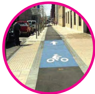
BIKE / VEHICLE CROSSING MARKINGS
